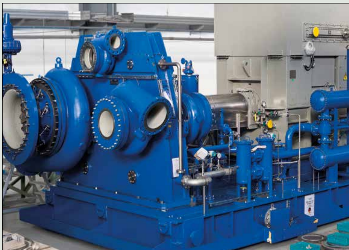
Siemens Energy has secured the contract to deliver and install its advanced centrifugal compressors for compressing hydrogen at Salzgitter. The compressor package features an integrally-gear design, allowing for more efficient compression
