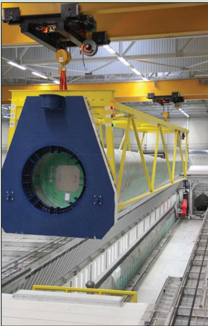
Blade production: blades are made of high-quality glass fibre-reinforced polyester. Source: Nordex SE
