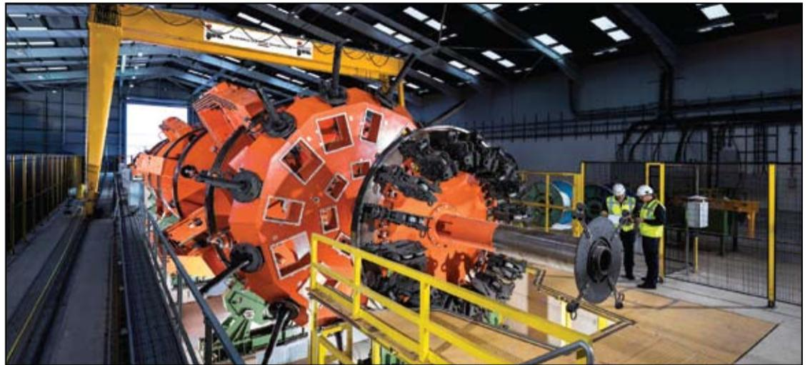
**JDR's new horizontal lay-up machine (HLM) machine. The HLM will enable JDR to provide the next generation of reliable and safe subsea connectivity to the oil, gas and renewables sectors**
