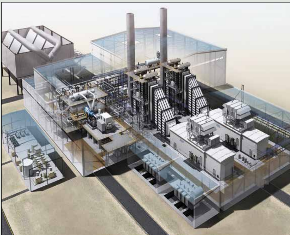
Artist's cutaway of an SGT-800 plant with batteries
