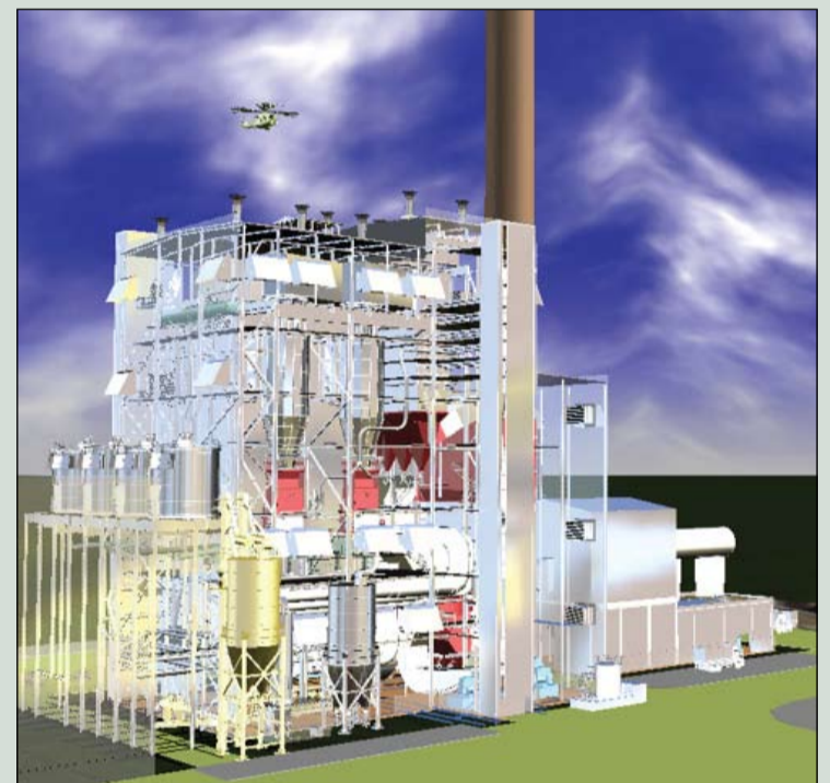
CAD cutaway of the 299 MW Tees Renewable Energy Plant biomass project. The project is being built on a brownfield site at the Teesport port facilities near Middlesbrough
