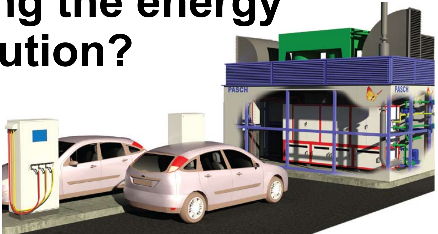
The COFAST project is based around the use of small-scale gas engines producing electricity for EV charging as well as heat
