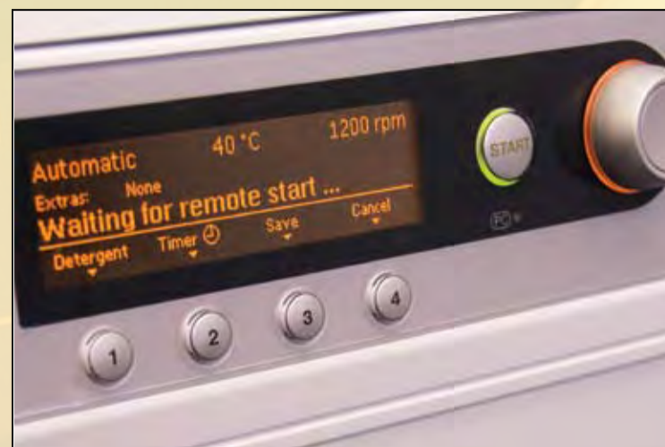
Off-the-shelf products have been altered to provide flexibility to the grid and allow coordination and control by the smart grid
