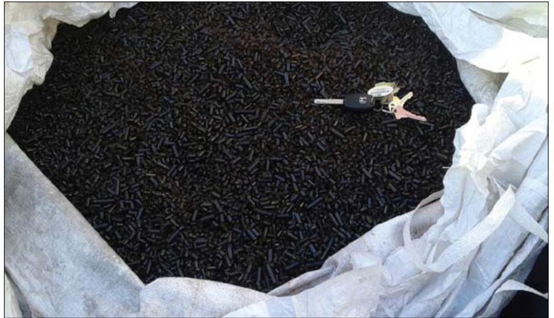
CoalSwitch is a 'black pellet' that can be ground into a very fine powder, capable of being used by coal handling systems and does not have the corrosive elements contained in biomass
