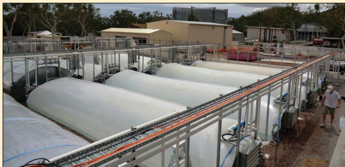
**Photo of the fully operational 10 m growth membranes producing oil-rich algae using the Tarong strain at MBD's R&D facility at JCU. The Tarong 1 ha plant will use up to thirty two 50 m membranes**
