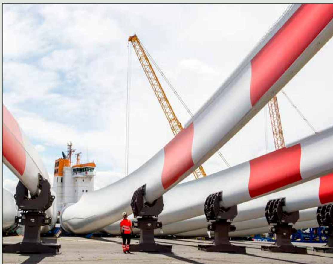
Siemens Gamesa RecyclableBlades leaving the blade factory in Hull (UK) for the Kaskasi offshore development (Germany)
