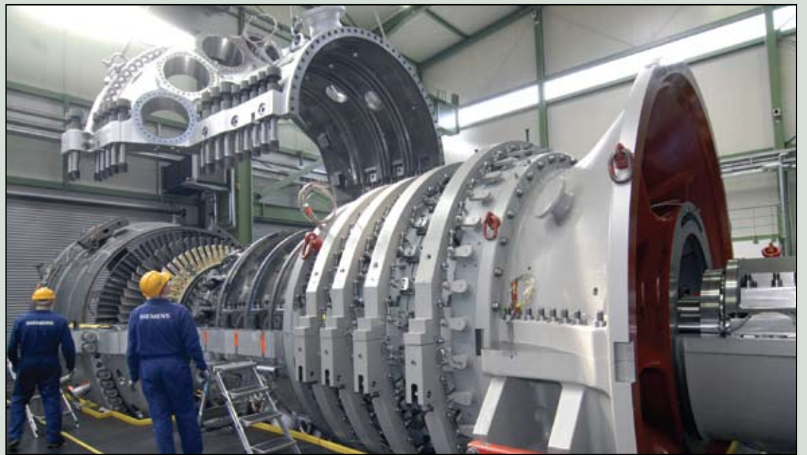
The gas turbine has 13 compressor stages and a four-stage turbine section
