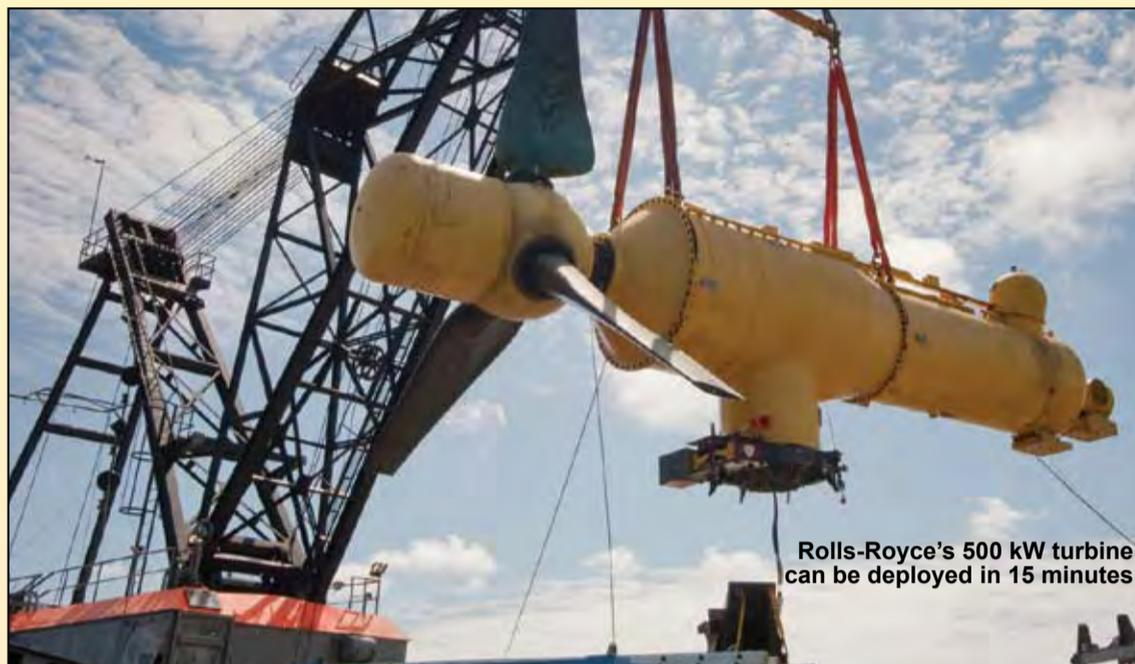
Rolls-Royce's 500 kW turbine can be deployed in 15 minutes
