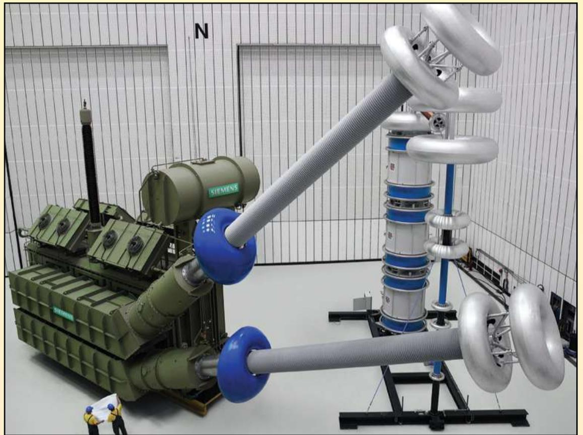
The 800 kV transformer in the factory in Nuremberg. It measures 26 m in length excluding the bushings
