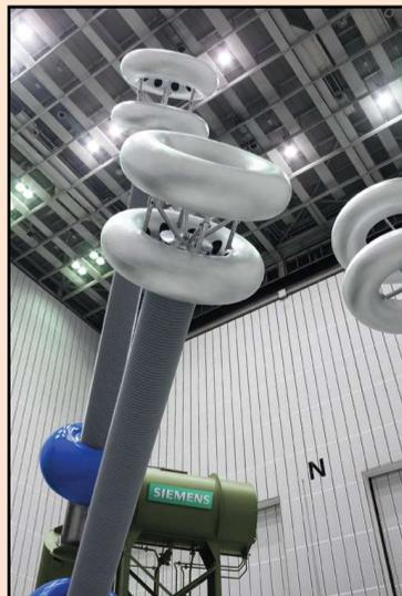
The two valve bushings, through which the current flows from inside the transformer into the converters, are 14 m long
