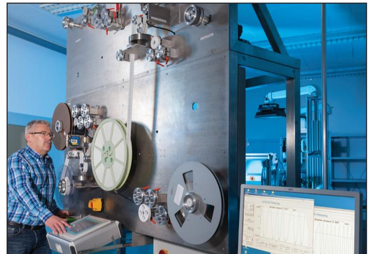
Ensuring that an embedded ceramic superconductor is precise to within one-one-hundredth of a millimetre when deposited on a substrate and coiled onto a bifilar winding © Siemens AG/Reprinted from Siemens' Pictures of the Future magazine
