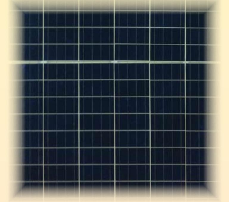
**Half cut cell technology essentially cuts traditional cell size in half so that modules can be made of 120 half cut cells with lower resistive losses and thus higher efficiency**
