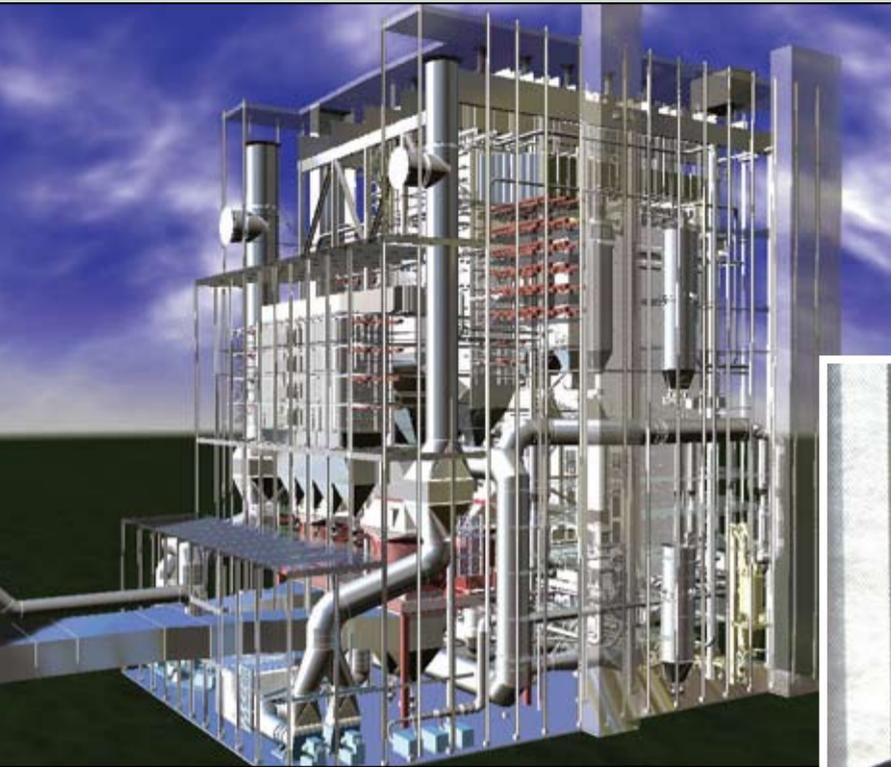
Cutaway of a single boiler
