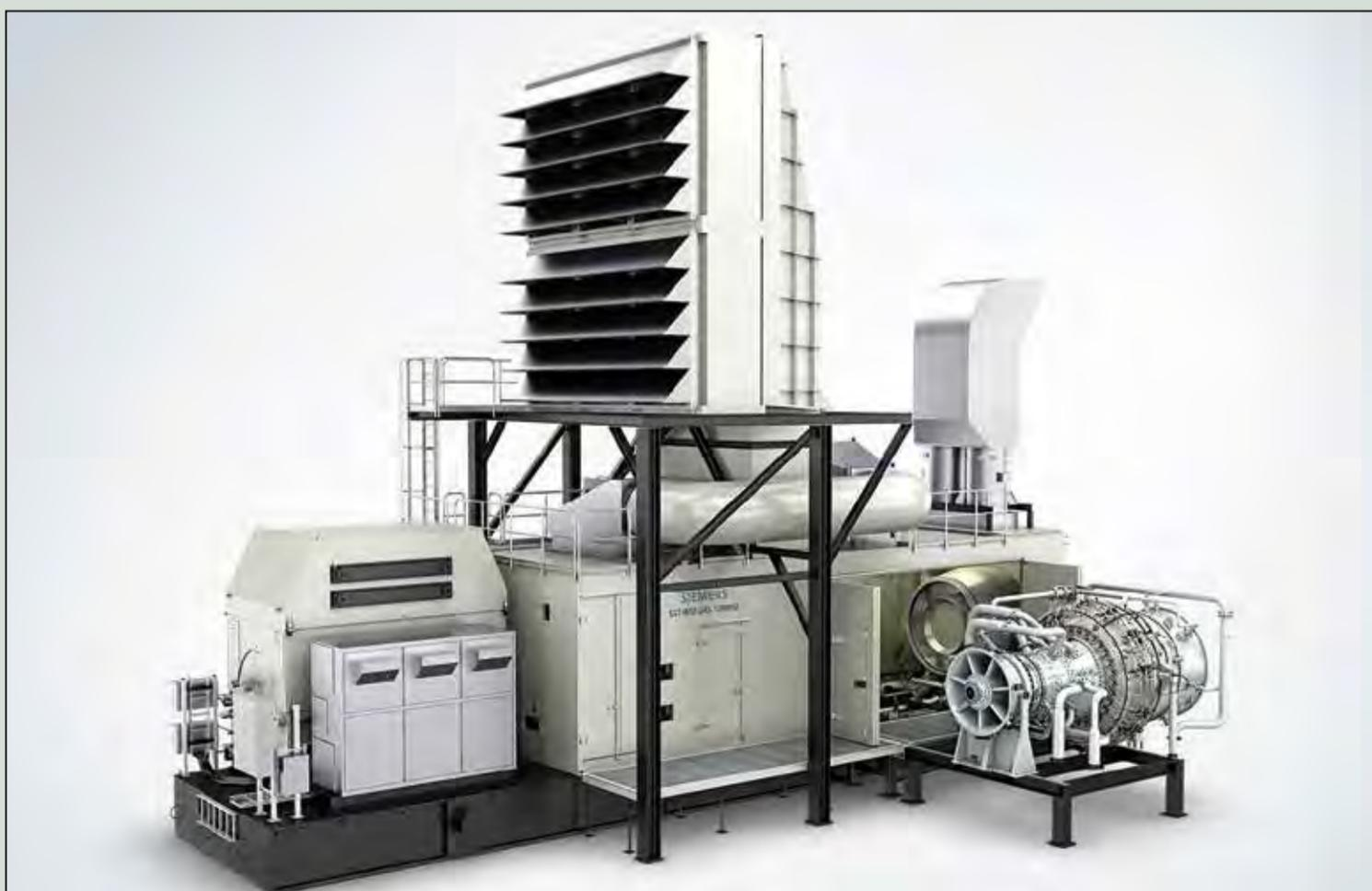
**The SGT-800 gas turbine will be provided as a single-lift package and 3-point mount installation, consisting of turbine, mechanical auxiliary systems, gearbox, generator and generator switchgear**
