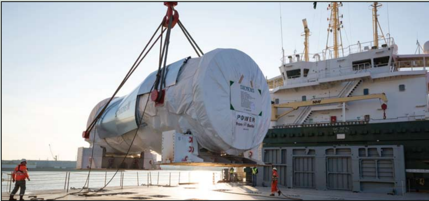
The first H-class gas turbine being loaded in Rotterdam on to a heavy load carrier before starting the journey to Egypt
