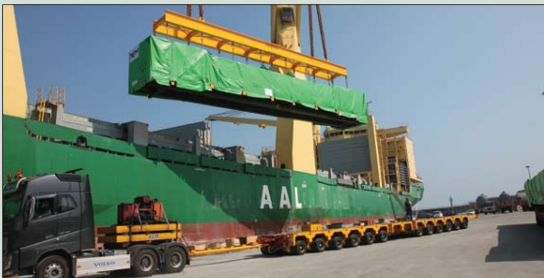
One of the HRSG modules for Beni Suef combined cycle power plant being loaded on to a vessel in South Korea
