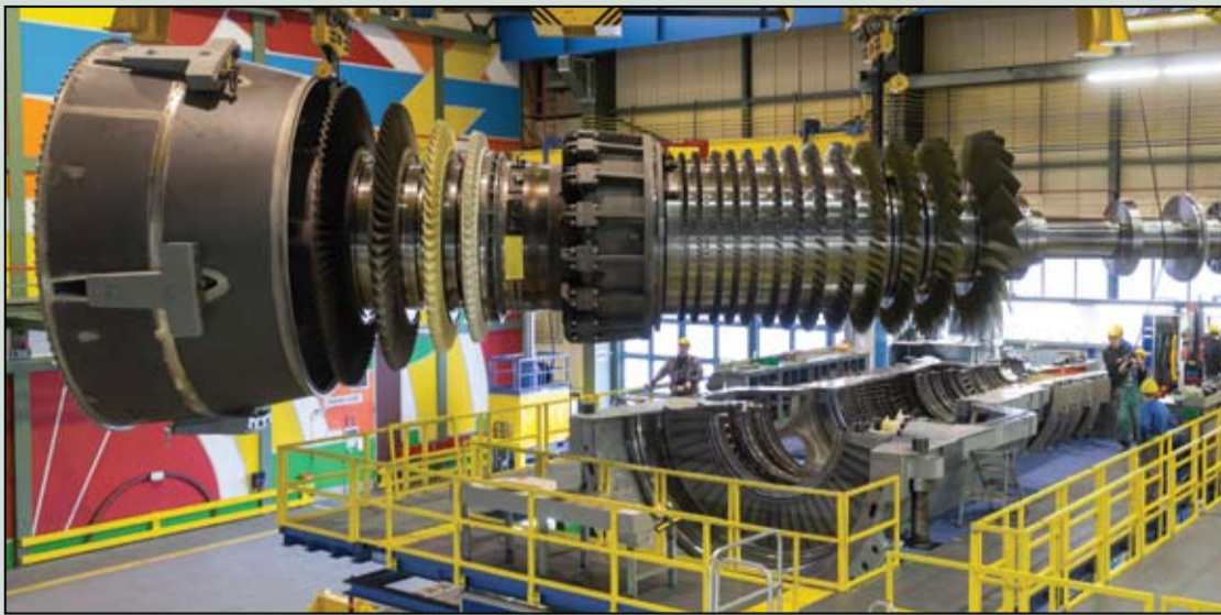
Turbine assembly: the SGT5-8000H has a four-stage turbine section and 13 compressor stages
