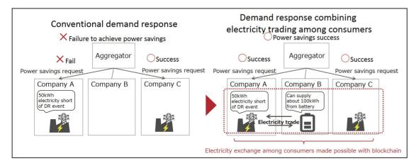
The system allows consumers to exchange electricity as part of a demand response scheme
