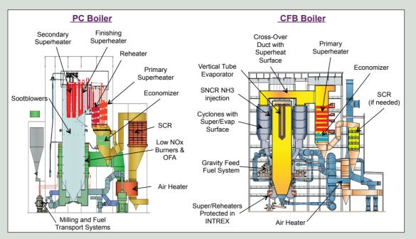
PC vs. CFB boiler design feature comparison
