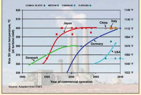
State-of-the-art in pulverised coal-fired power plant steam temperature
