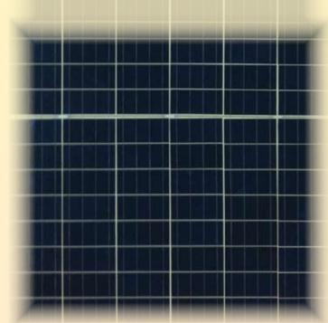
Half cut cell technology essentially cuts traditional cell size in half so that modules can be made of 120 half cut cells with lower resistive losses and thus higher efficiency
