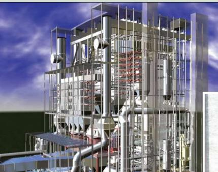
Cutaway of a single boiler
