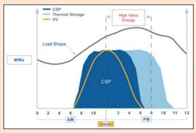
Matching CSP electricity production to peak pricing periods, due to the use of thermal storage
