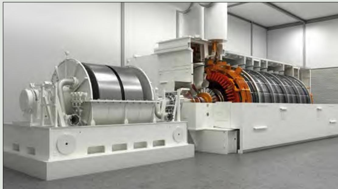
**To provide maximum inertia, synchronous condensers solution can be extended with additional rotating mass from a flywheel**
