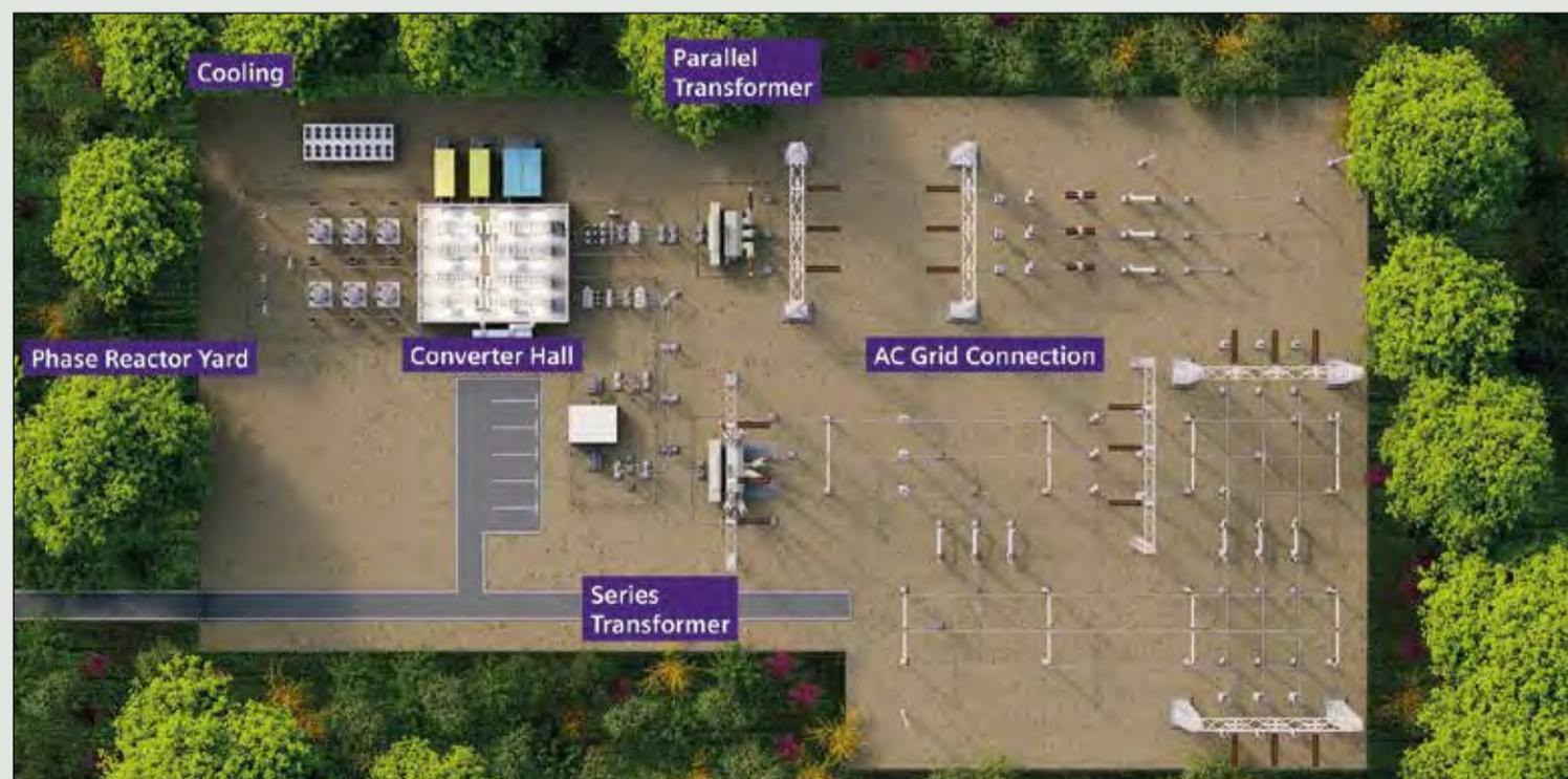
Aerial view of various components in a typical UPFC PLUS system
