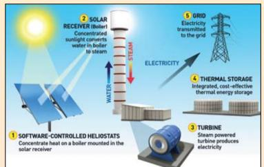
At full capacity, Ivanpah's three solar towers produce a gross total of 392 MW of solar power. The project uses 173 500 of BrightSource's heliostats
