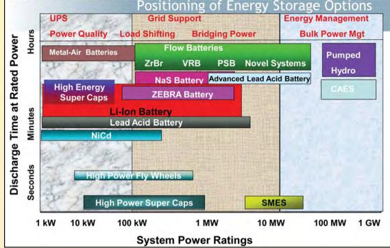
There are a number of technology options for energy storage, each operating in different power capacity ranges. Source: EPRI and Saft
